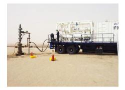
Haimo <u>High Performance Tester</u> (HPT) is an excellent tool for field verification of meters including MPFM.
